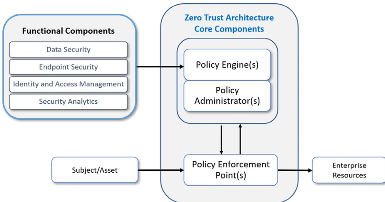
Figure 2: ZTA High-Level Architecture
